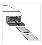
Push the module into either of the slots—it doesn't matter which one—until it is fully inserted; the button to the right of the slot will pop out. Ensure that the CAM is the correct way up; the multi-way connector should be pushed into the slot, and the corner of the connector that does not have a small plastic ridge sticking out should be at the top left.
